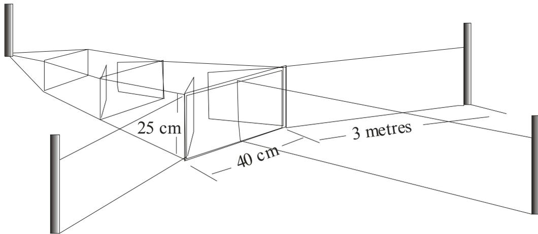
Figure 2. Design of the fyke net.
