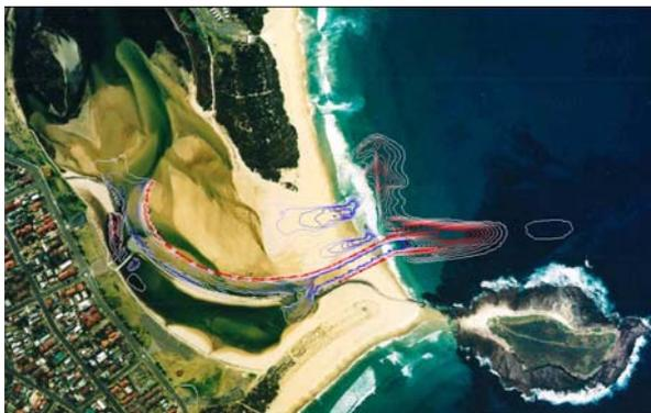
**Figure 8:** Option 6 bed change over first 36 hours of 100 Years ARI flood.
